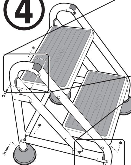
Insert (2) bolts through frame elbows and secure with (2) nuts. Insert (4) casters, aligning holes in casters with holes in frame. Attach with (4) bolts and (4) nuts. Tighten all nuts securely.
