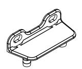
1. Lay the drawer sides down on flat surface. <u>Carefully line up</u> the drawer bracket with the holes in the drawer side as shown. Using a hammer, tap each drawer bracket stem part way into each hole. Repeat this process until the drawer bracket is fully seated in the drawer side.
