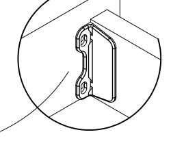
1. Notice, the drawer bracket holes are slotted. Drawer fronts can be adjusted by loosening screws, making needed adjustments and retightening screws.
